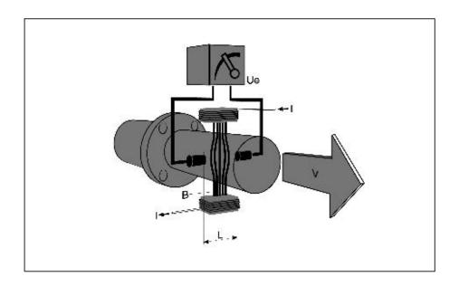
Ue = B - L - v Q = A - v Ue = 感应电势 B = 磁场距离 V = 流速 Q = 体积流量 A = 管道横面
